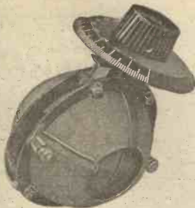
A photograph of the "Varic" variometer made by Messrs. Lionel Robinson and Co.
