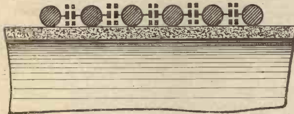
Fig. 1.—Illustrating the capacity effect between the adjacent turns of a coil.
